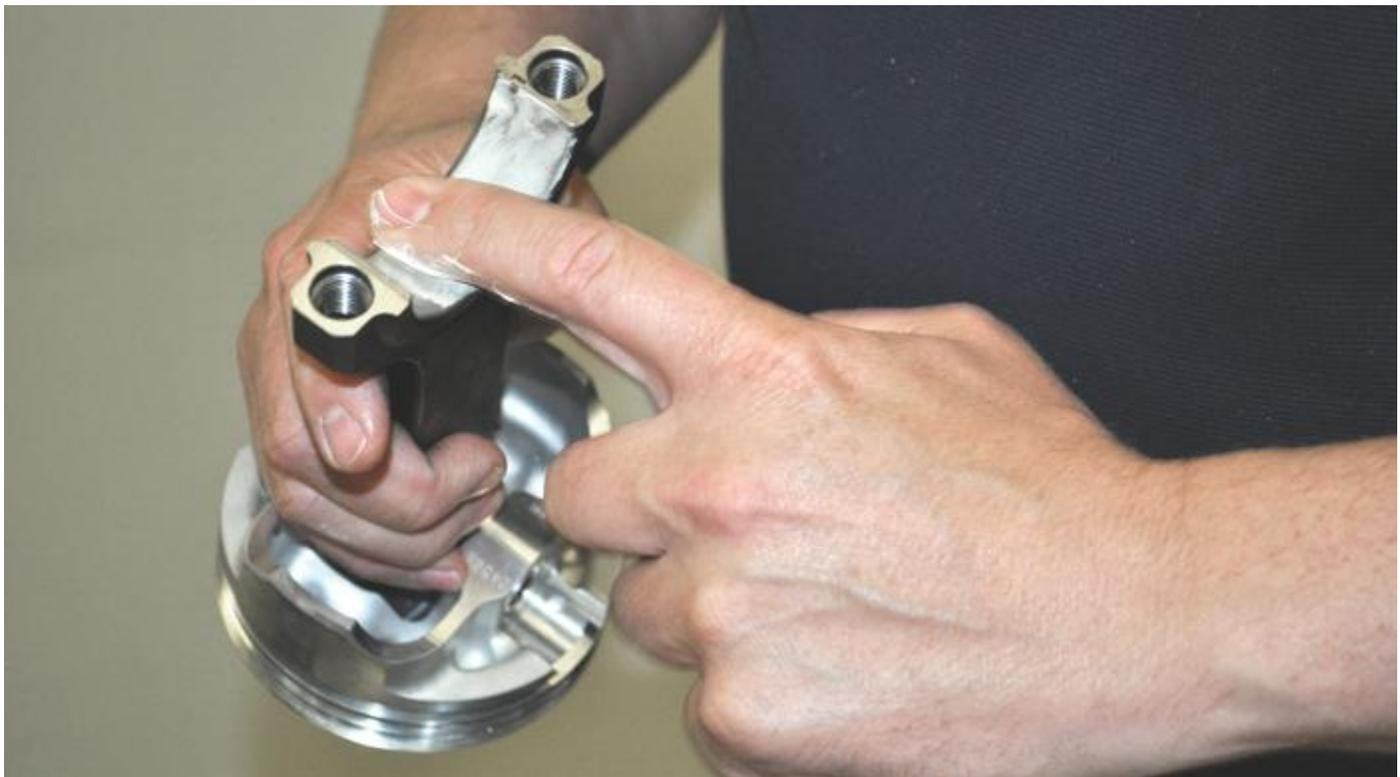
*A thin coating of assembly lube should be applied on all high-friction, high-load surfaces including rod, main and cam bearings.*
